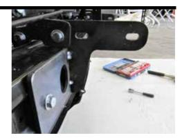
Install rear mounting bracket to front mounting bracket at top using two (2) M10 x 40 bolts. In lower hole of rear mounting bracket fit one M10 x 85mm bolt, flat washer, spring washer and nyloc nut.
